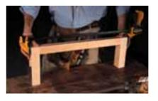
Be sure to make a full-size mock-up of the legs and sides to determine the angle you need to cut on the bottom of the legs.
