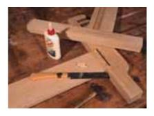
Peg the tenons that join the front rail to the front legs and the back rail to the back legs. If you've ever pegged tenons before, you know that dowels can be wildly different sizes than they're supposed to be. Here's a trick. If your dowel is a bit undersized, glue it in place and cut it nearly flush to the surface. Then put several drops of thinned glue on the end grain of the dowel. It wicks in the glue, expands and glues up tight. When the glue is dry, cut the dowel flush.
