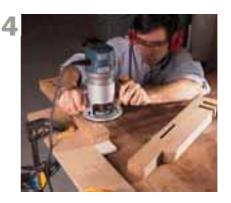
When pattern-routing the curve on the legs, make sure you have the work firmly clamped in place. I have the pattern and leg wedged between two pieces of oak (the pattern is on the underside of the leg). Then the leg itself is clamped to the table. You also could perform this operation on a router table with a starting pin for pattern-routing.
